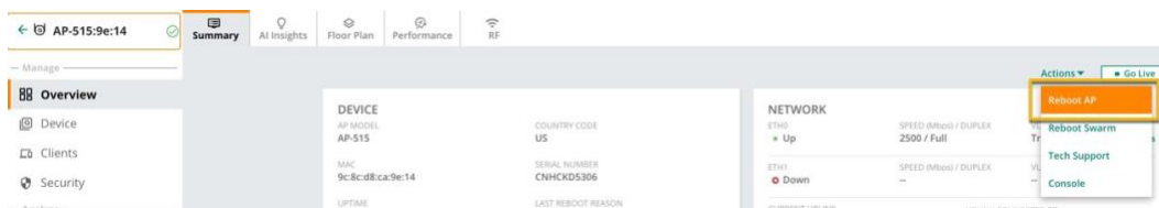
Figure 51 Rebooting Teleworker's IAP
